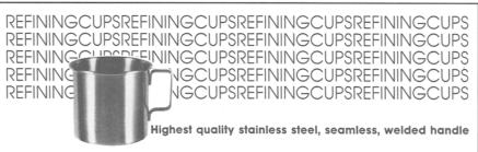
Used in conjunction with AOCS Official Method Ca9a-52 to determine the refining loss of free fatty acids, oil and impurities when the sample is treated with alkali solutions under test conditions. The method applies to crude peanut oil, crude coconut oil, crude corn oil, crude soybean oil (expeller and hydraulic), and crude cottonseed oil (expeller and hydraulic). Cup dimensions: 4 1/2 inch diameter and 4 1/8 inch depth. Capacity: 960 ml.
